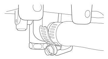
15. Loosen hose clamp with a flat head screwdriver or a 5/16 socket wrench to remove hose from jet.
